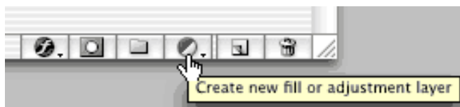
Figure 8: Create a New Adjustment Layer by choosing it from the Layers palette pop-up menu.
