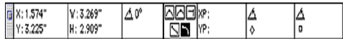
Figure E: The Measurements palette provides quick access to nearly all properties associated with points and segments.
