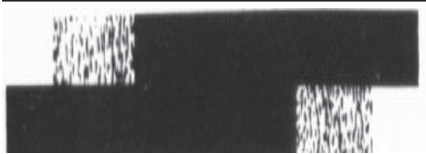
Scale indicating Over exposure, or a correct reference point for bold copy with off-white or soiled background.
