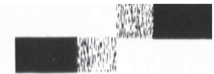
Scale indicates under exposure or weak developer, or is correct reference point for weak copy or very fine lines.
